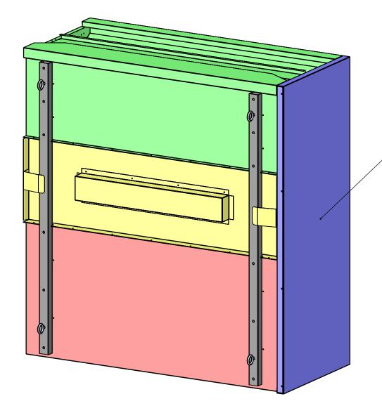
If one of the sides of the hood module is either at the right \_\_or left extremity of the hood, you need to install the corresponding side panel to this side
