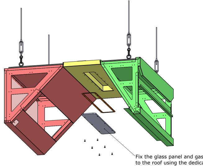
Fix the glass panel and gasket to the roof using the dedicated 6 glass screws with special washers
